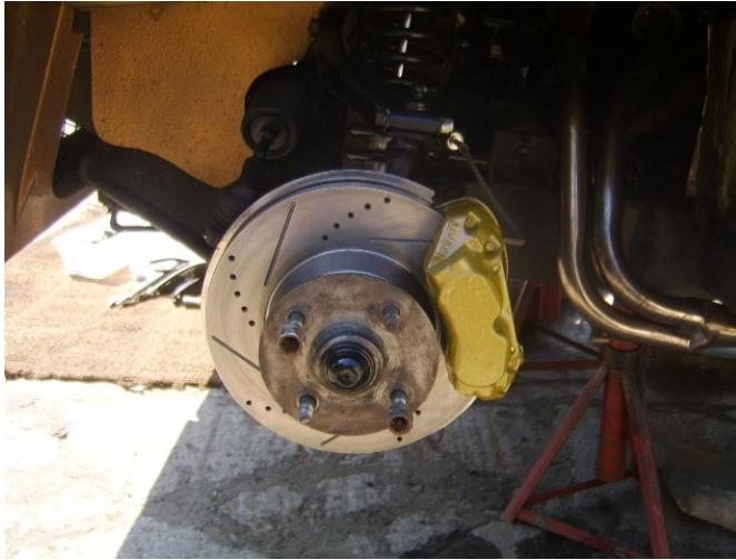
The Jaguar Brake Set Up on MB33
